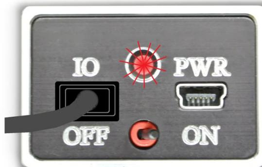
5. Following the flashing red the LED should become a steady green.
