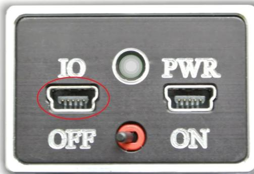
4. Turn the nanoMCA ON. The red LED should be flashing quickly for about 15 seconds.
